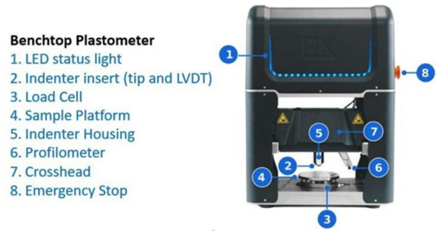
Fig 1. The PLX-Benchtop and its components.
