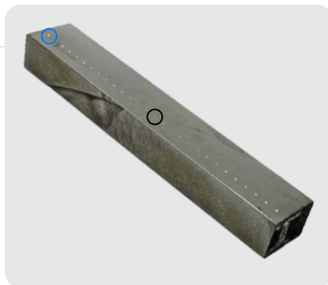
Figure 1: A hot-rolled high-strength steel beam was PIP tested, revealing property differences between the edge and centre.
