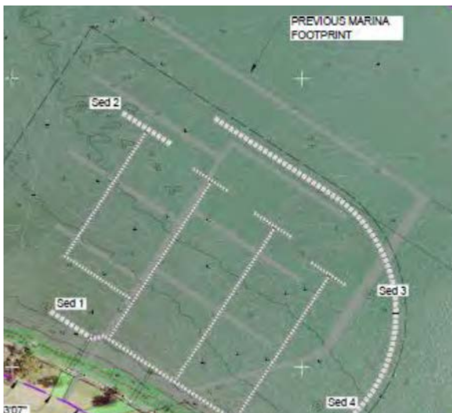
Figure 2 Extract from CEMP (Ref [1]) identifying sediment 'impact' locations.
