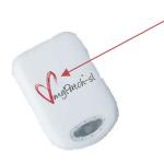
Tap twice in the middle of the myPatch®-sl ECG Recorder to mark an event during the recording period. A solid BLUE light will come on briefly to acknowledge the recording of the event.
