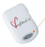
To end the recording, hold down the power button on the bottom of the myPatch®-sl Recorder for 4 seconds, you will see a **RED** light come on indicating that you are ending the recording. Then you will remove the myPatch®-sl Recorder from the Electrode and set aside.
