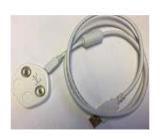
MAKE SURE the myPatch®-sl Holter Recorder is fully charged. Connect the myPatch®-sl Recorder to the myPatch®-sl USB Transfer Cable. Do not force the myPatch®-sl ECG Recorder onto the connection of the cable, it will only snap on in one direction. Then connect the USB-end of the myPatch®-sl USB Transfer Cable to a powered on computer or provided wall charger.
