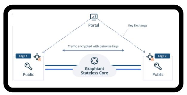
The payload is encrypted edge-to-edge, with only the Edges able to encrypt and decrypt it. With no edge-to-edge tunnel, there's no need for a full session state or running BFD or IP SLA probes. Compared to an IPsec relationship, our approach is quicker to set up. In a full mesh environment with transport flaps, many tunnels terminated on each edge increases this time exponentially.
