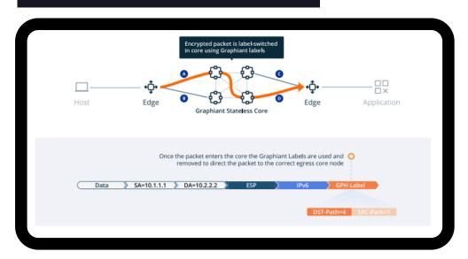
Once the packet arrives at the Core node servicing the destination edge, it adds an integrity protection header before forwarding to the final edge. The edge can then determine the source, understand the header information, and use its private pairwise encryption key to open the payload.
