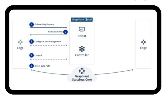
Our software never generates keys. Instead, we rely on TPM or HSM and use private/public keypair for setting up primers and symmetric encryption keys. The keystore resides on the device HSM and is under the customer control. Graphiant never accesses the private keys and doesn't use preshared keys.
