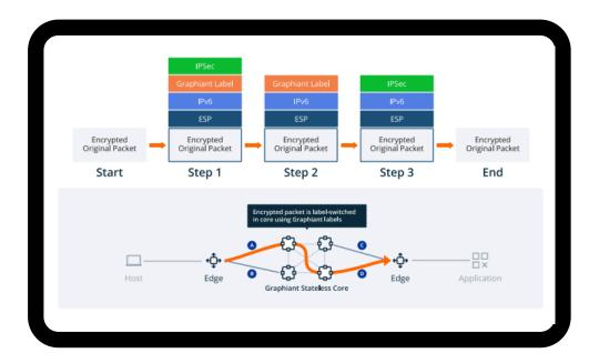
As packets from the LAN enter the Graphiant Edge, we first encrypt the packet and add ESPv3 header based on established security association (SA). The Edge does not build a full IPsec tunnel end to end; separating each is crucial.
