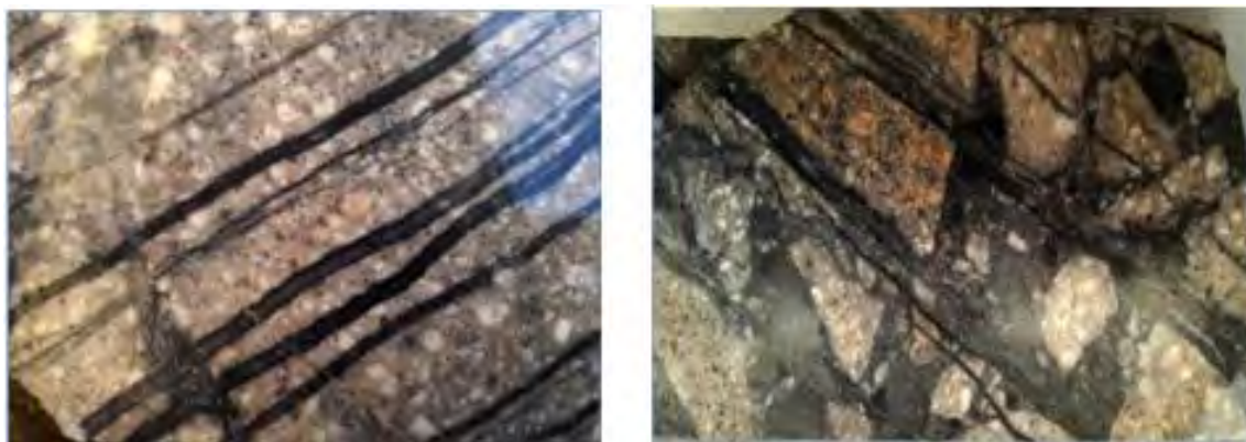
(a) (left): Sheeted 1 to 3 mm wide V2 micro-veinlets cutting the feldspar porphyry in AP-23-297 at 228 m depth. (b) (right): Sheeted 1 to 3 mm wide V2 micro-veinlets cutting the Polymictic Breccia in AP-23-297 at 222 m depth.
