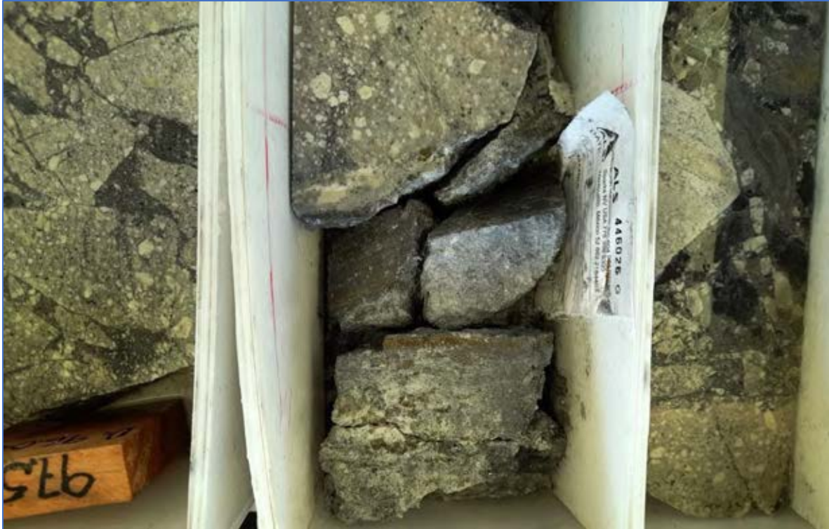
3 cm wide zone of clay-rich fault (bottom of center row of core) with disseminated pyrite within the Polymictic Breccia. From AP23-297 at 98 m depth; photo of PQ core; width of core is approximately 8.65 cm.
