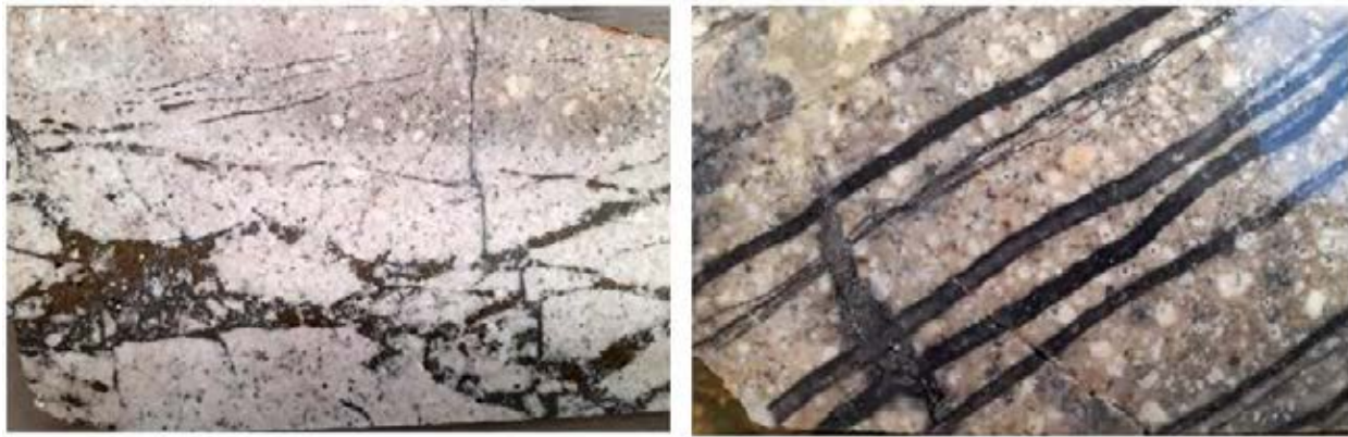
(a) (left): V2bx micro-veinlets dilating to form a local breccia zone. From AP-23-303 at 30 m depth.
