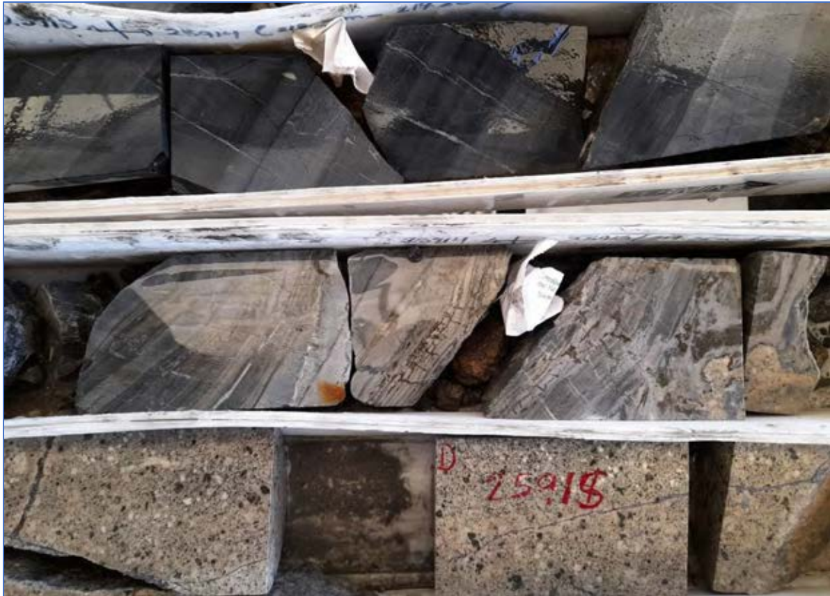
Thin-bedded sediments altered to hornfels at the contact of a feldspar porphyry grading out to almost fresh limestone-shale sediments. From AP-11-80 at 215 m depth; HQ core with width of core of approximately 6.35 cm.
