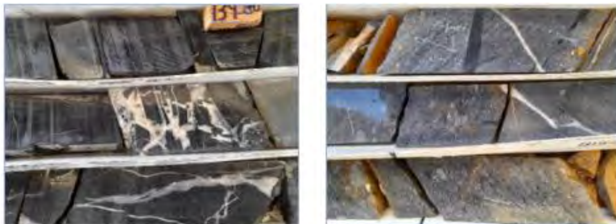
(a) (left): thin-bedded calcareous limestones and shales and one thin ash tuff (bottom row, center). From AP-15-250 at 140 m depth. (b) (right): bedded lapilli tuff from AP-13-170 at 31 m depth. HQ core (top to bottom field of view) of approximately 6.35 cm.
