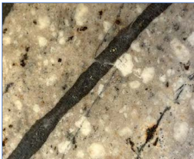
3 mm wide sheeted V2 micro-veinlet with visible gold flakes down the center and cutting the feldspar porphyry in AP-23-303 at 206 m depth.
