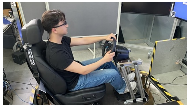
Figure 3: Driving Setup with an adjustable chair, pedals, steering wheel and a person wearing eye tracking glasses
