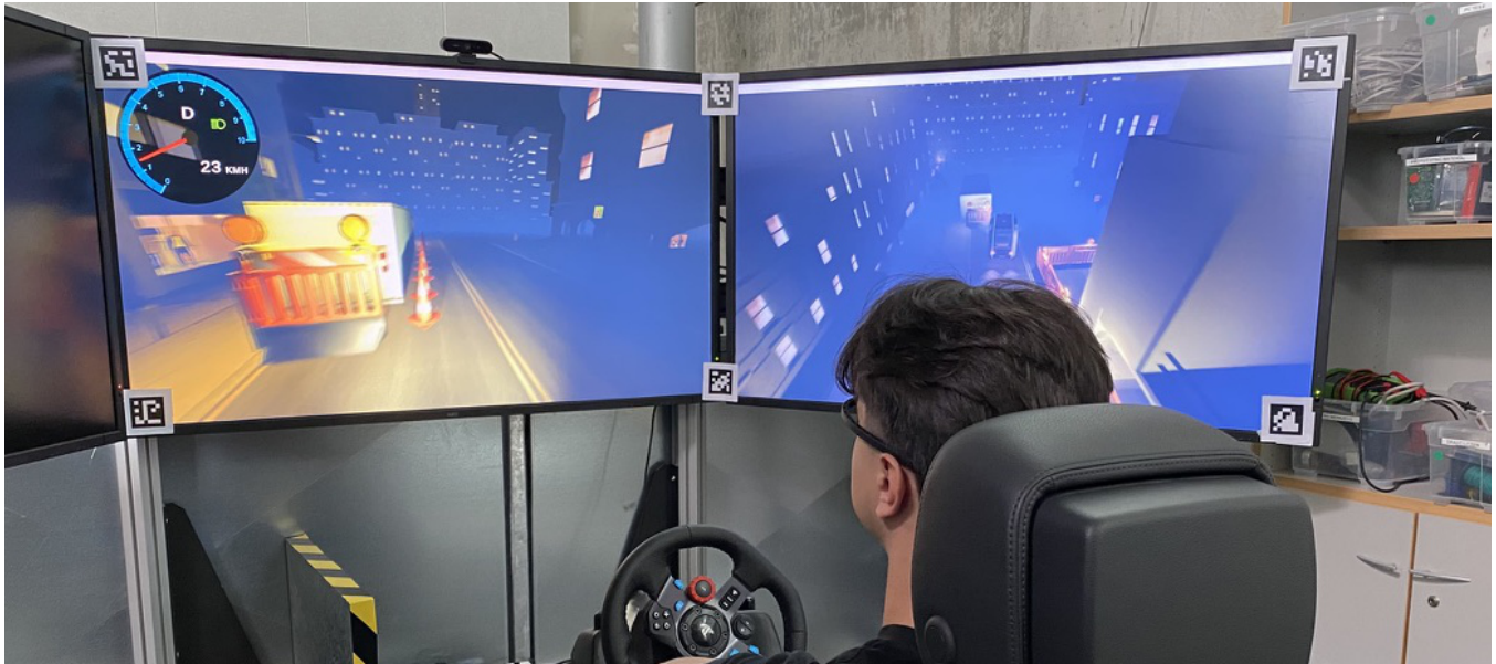
Figure 1: Driving simulator setup with the participant seeing the front view in the center and the uav view on the right.
