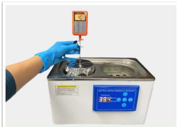
Place agarose solution into hot water bath (37-40°C)
