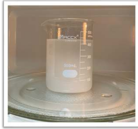
1. Heat dissolved agarose solution in microwave
