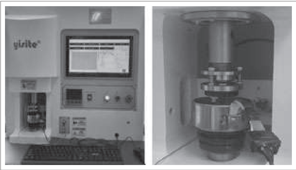
Figure 4. The EMMW-1W tribometer used for measuring friction and wear of contact pairs under dry or lubricated sliding conditions, installed in the Mechanics Laboratory (“Model EMMW-1W...” 2025).
