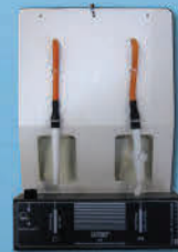
WT1 Psychrometric kit dry and wet bulb
