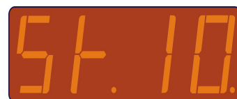
Input Condition Example showing step 1 for input 1 & Step 0 for input 2 ( tTYPE =1)
