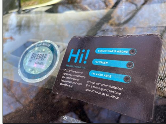
Figure 3: Exterior of Evo Car Share Toyota Prius + NFC card reader and availability indicator
