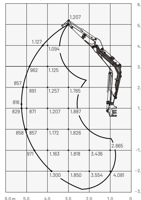
The loads in the diagram are within 87% of the hydraulic lifting load and within 75% of the tipping load.
