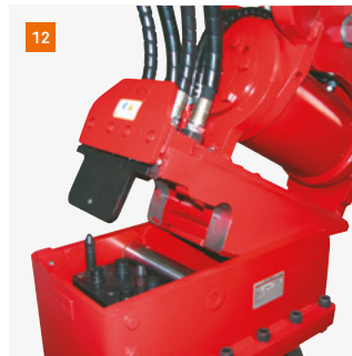
12 HUPPQuick system: Hydraulic connections are connected automatically during the quick coupling process
