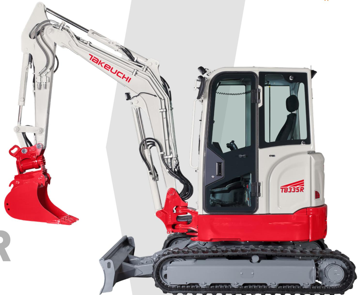
The **TB335R** short tail excavator is characterised by its minimal rear overhang. Thanks to its compact design, our 3.9 tonne excavator is easy to manoeuvre without losing stability. Especially on hard-to-reach construction sites and in urban areas the TB335R is your closest ally. Equipped with state-of-the-art technology and a new, very well-equipped cabin with intuitive features, the TB335R offers you a modern and comfortable workplace for maximum productivity and performance.
