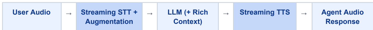
Figure: Optimized streaming cascade. Each stage begins processing before the prior stage completes. The augmented STT layer passes emotion, prosody, and behavioral metadata alongside the transcript, giving the LLM the full conversational context.
