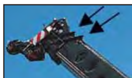
A-max extends only the inner-mid section of the boom for substantially increased capacities for in-close, maximum capacity lifts.
