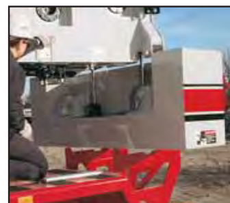
Fast & efficient hydraulic counterweight removal enhances roadability
