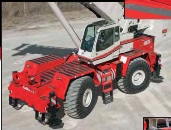
Fast & efficient hydraulic counterweight removal enhances roadability
