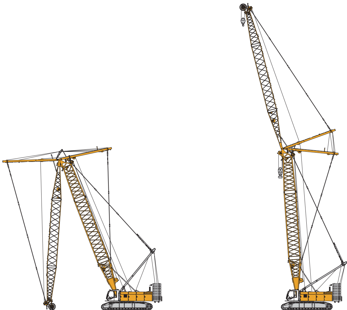
Erecting of main boom and luffing jib
