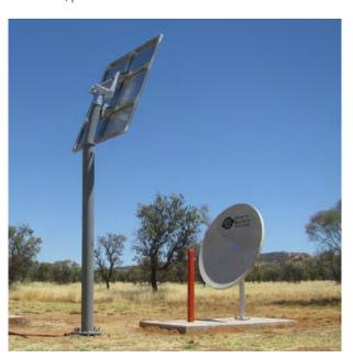
This location is over 100km from the nearest mobile phone radio base station, extending access to a useable mobile phone signal almost ten times further from the tower than normally experienced.
