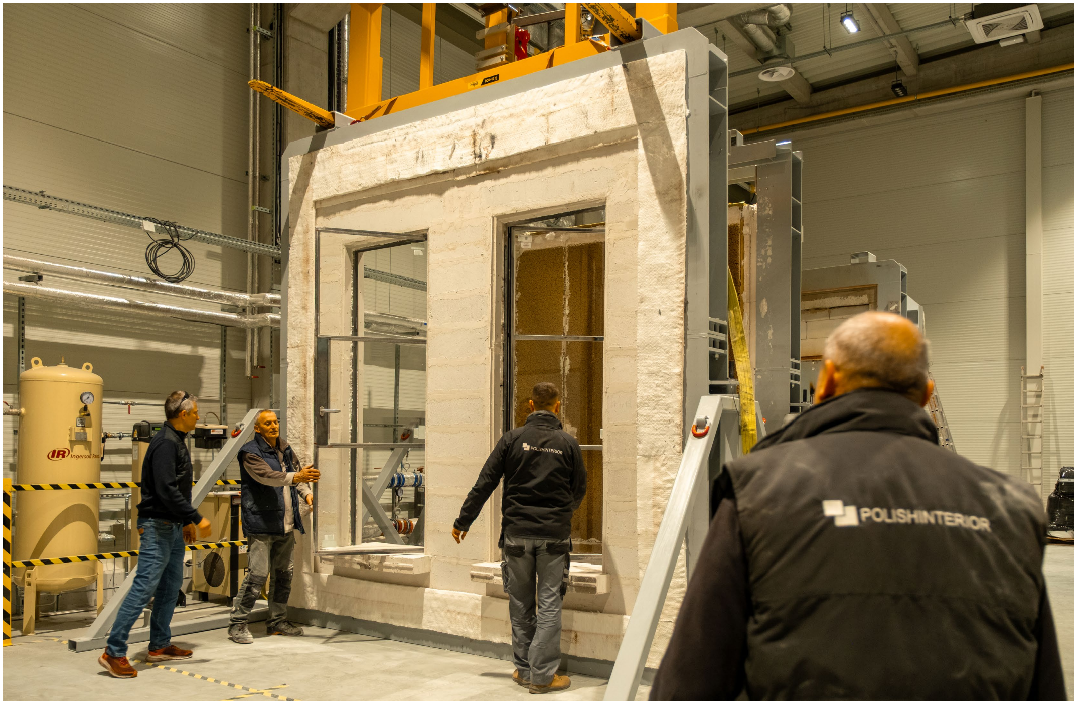
Pioneering safety - our industry-first fire-rated steel doors undergoing rigorous testing, setting new benchmarks for performance.
