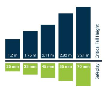
Safeplay Fall Protection Sheets are installed on a sand foundation of approximately 20 cm. In combination with the specially designed artificial grass Playgrass 24 or Playgrass 24 Recycle (both available in several unique colors), the Safeplay System ensures perfect drainaige, excellent stability and the required HIC-values. After installation, the artificial grass is filled wit silica sand 0.3 - 1.0 mm (approximately 25 kg/m²) for a durable and wear-resistant surface.
