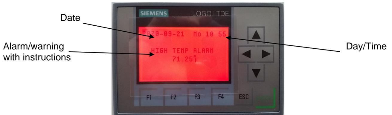
When a Warning or Alarm occurs, the screen will change color, Orange for a warning and Red for an alarm. The condition of the unit will be displayed, along with the time of the event and recommended resolution.
