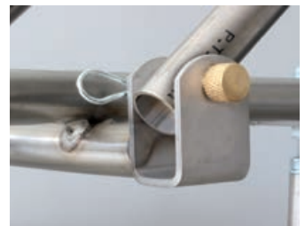
transportable: easy disassembly
