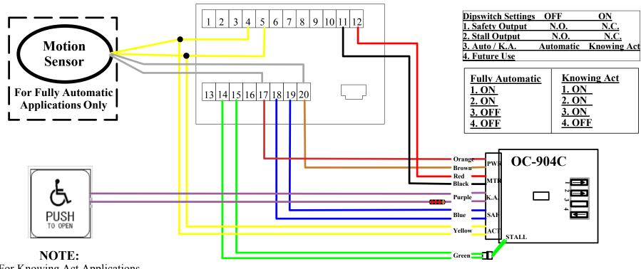
For Knowing Act Applications all activation devices must connect to the purple wires from the OC-904 control (N.O. Dry Contact Only.) Push/Pull activation must be DISABLED at the door control.
