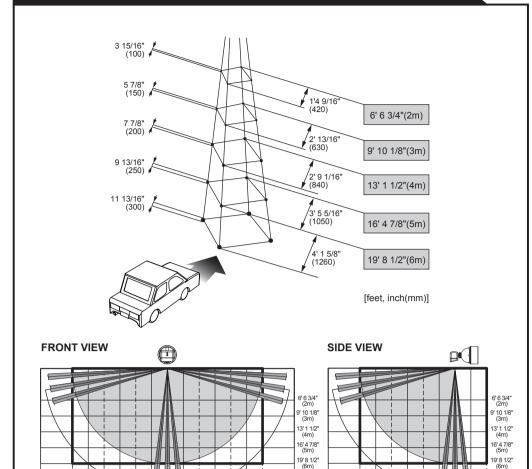
NOTE The actual detection area may become smaller depending on the ambient light, the color / material of the object or the floor as well as the entry speed of the object.
