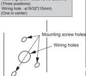
⚠ CAUTION : Risk of product failure. Do not install sensors upside down. Otherwise rain water makestroubles 0 Right position of the nounting screw holes wher 0 0 install on the side pole Right sensor position whenuse a angle. Make sure to remove burr in mounting holes otherwise
