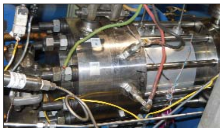
Figure 1: A supercritical CO 2 turbine-alternator-compressor operating at Sandia National Labs
