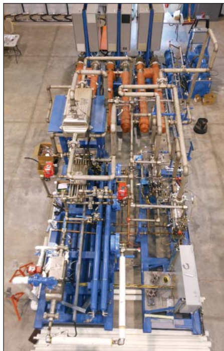
Figure 4: Sandia's S-CO 2 test loop
