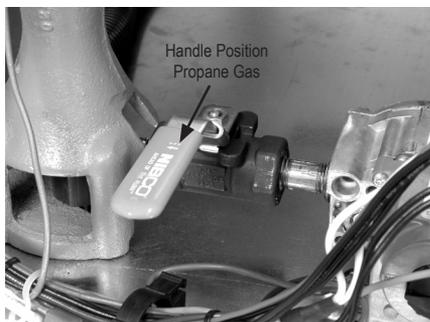
3. The handle must be fully set at 90 degrees to gas flow (propane gas) or parallel to gas flow (natural gas) for proper operation. Also refer to the decal located on the heater's base, adjacent to the selector valve.
