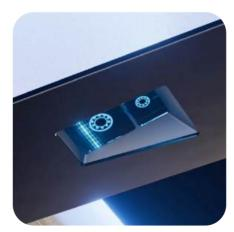
The system is based on **real-time body detection** in 3-D virtual environment and high-quality imaging (10 fps, precision +-1mm).
