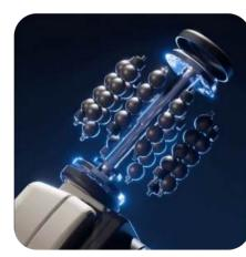
It uses collaborative robot and a complex pneumatic system to apply pressure with special vibrocompression massage tool (100-450 rpm, 120 to 540 Hz).
