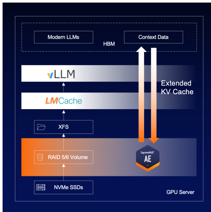
Conceptual reference architecture for SupremeRAID™ AE KV cache offload
