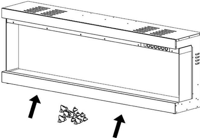
4. After placing the fuel bed media, fasten screws back on the glass panel.
