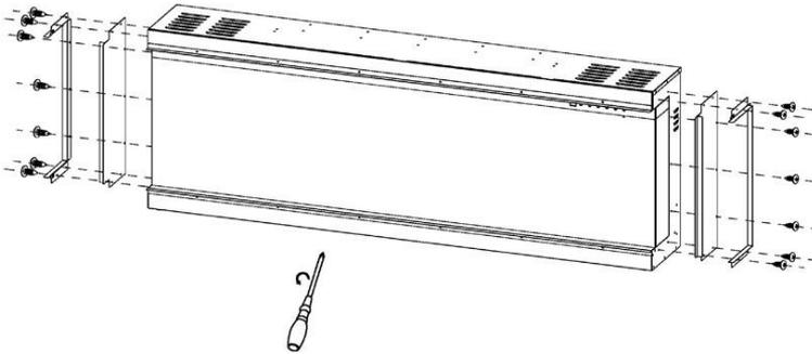
4. Remove the screws from the fireplace as shown in the picture below.
