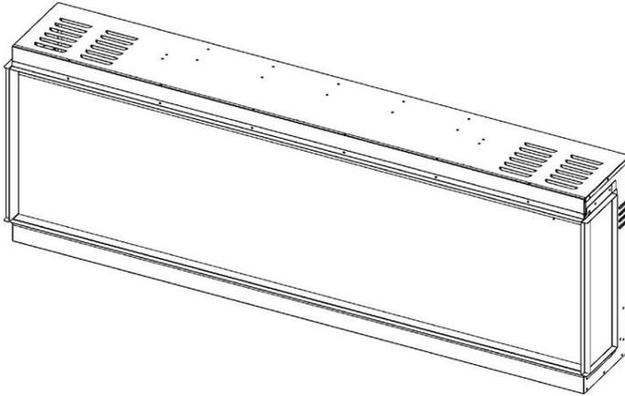
2. Remove the 7 screws on the right side. Take off the fending bar and panel.
