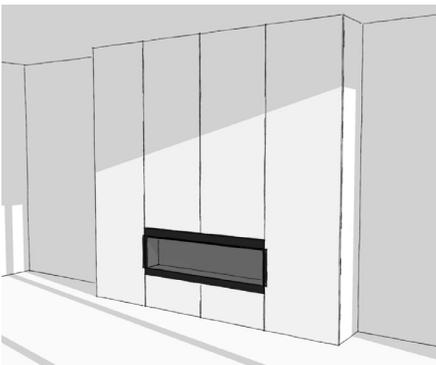
Insert the fireplace into the wall opening and align to the finished wall lining. Fix in place through the side brackets. Protect the glass panel until completion.
