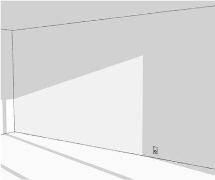
Find a suitable location with an electrical outlet within **1m** of the fireplace.
