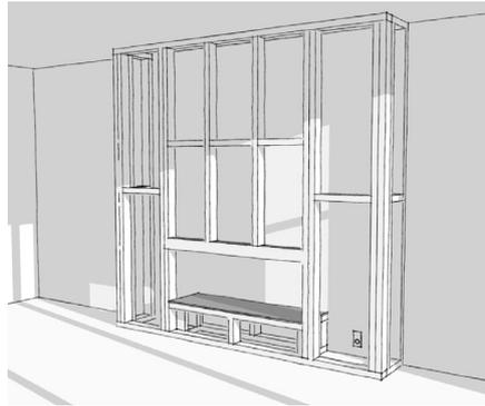
Construct the cavity to the desired size, allowing for the following wall opening dimensions: **1250W x 435H x 254D mm**
