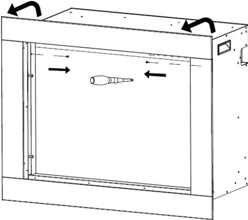
2. Use a screwdriver to take off the FOUR screws shown below. Remove the glass panel and move it to a clean, soft place to avoid scratching it.
