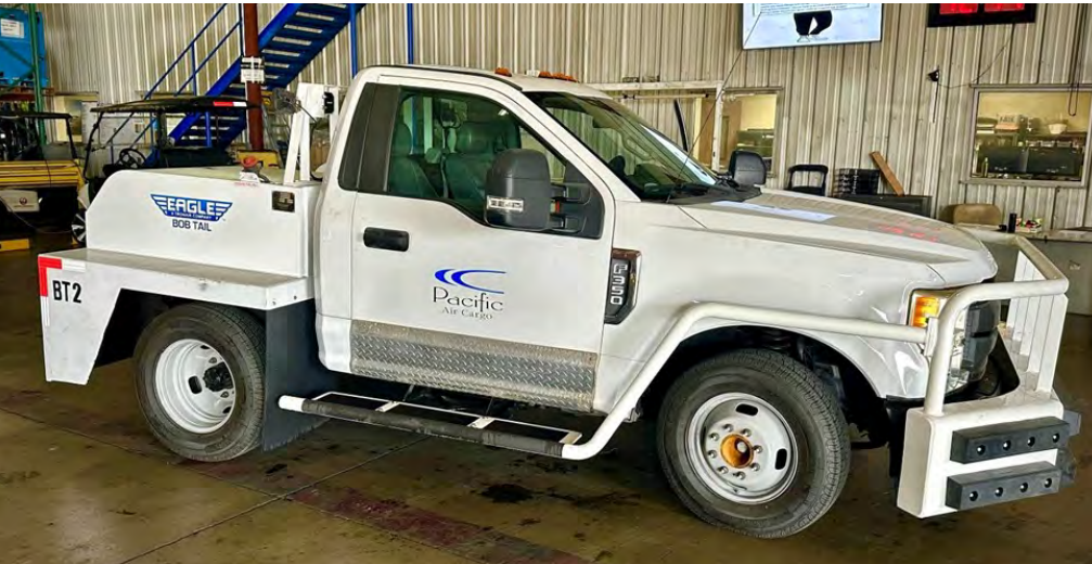
TB-1 and TB-2, 10,000 lb. DBP joins our PAC family of tugs as the heavy and fast pullers in the bunch.
