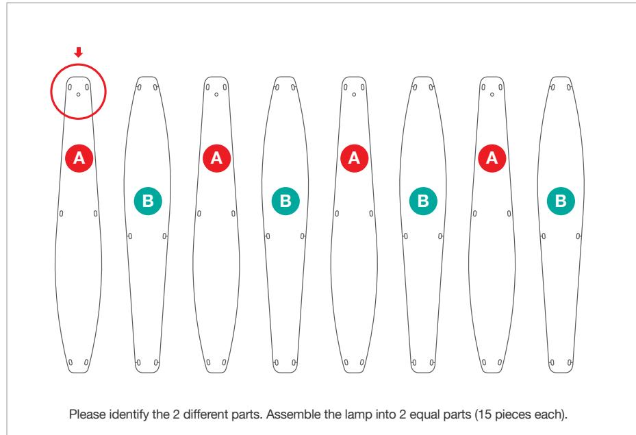
Please identify the 2 different parts. Assemble the lamp into 2 equal parts (15 pieces each).
