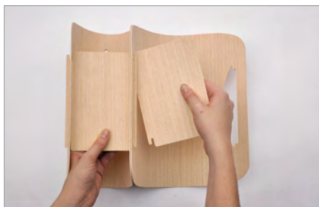
9. Repeat previous steps. Always assemble next part behind previous part.
