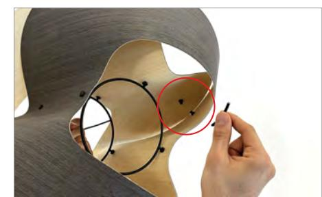
12. Take one of the metal wires and insert it into the rubber bands inside the lamp.
