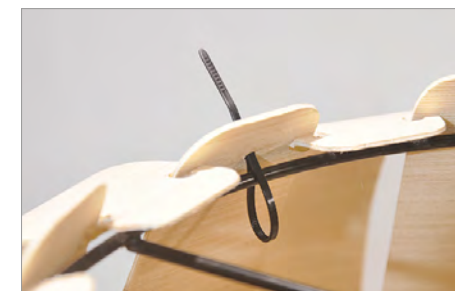
7. Join A wood hole with metal ring with PLASTIC SEAL.
