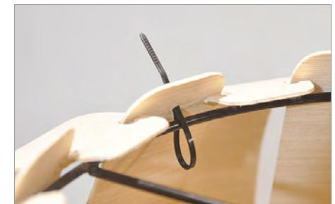
7. Join C wood hole with metal ring
