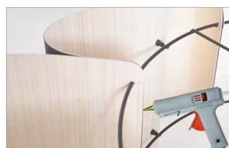
11. Once assembled, we suggest to stick mating parts nodes with adhesive for wood.
