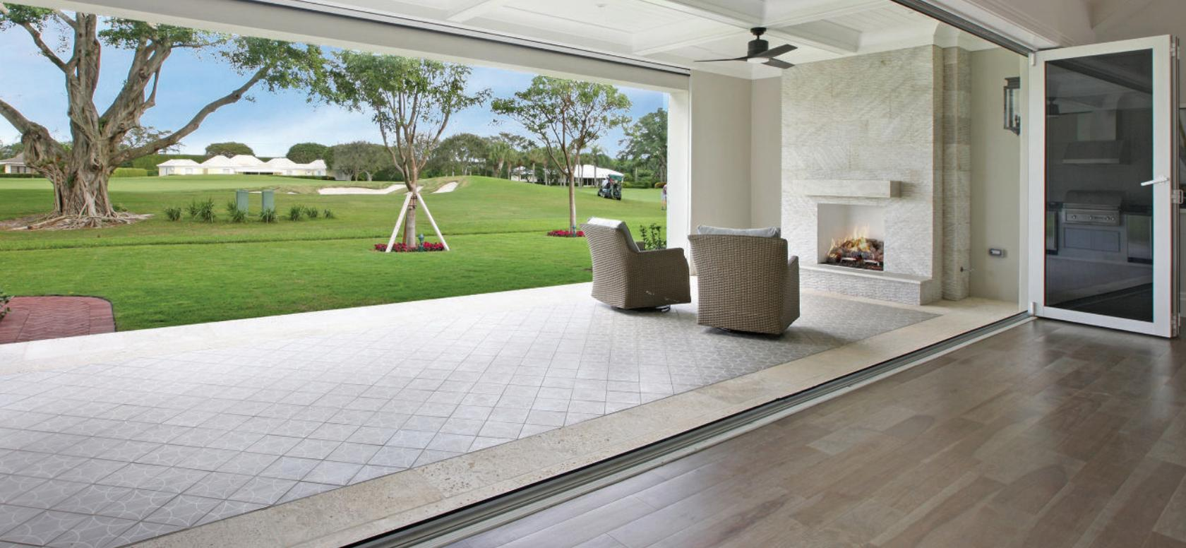
The thermally broken Vista Fold™ aluminum door system provides unobstructed views and seamless transitions to the outside. Euro-Wall thermally broken folding doors systems can span heights up to 168”, widths up to 52”, can be configured as a radius or postless corner systems and can span any opening width with an unlimited number of sequential panels. Vista Fold™ applications are Florida Product Approved.
