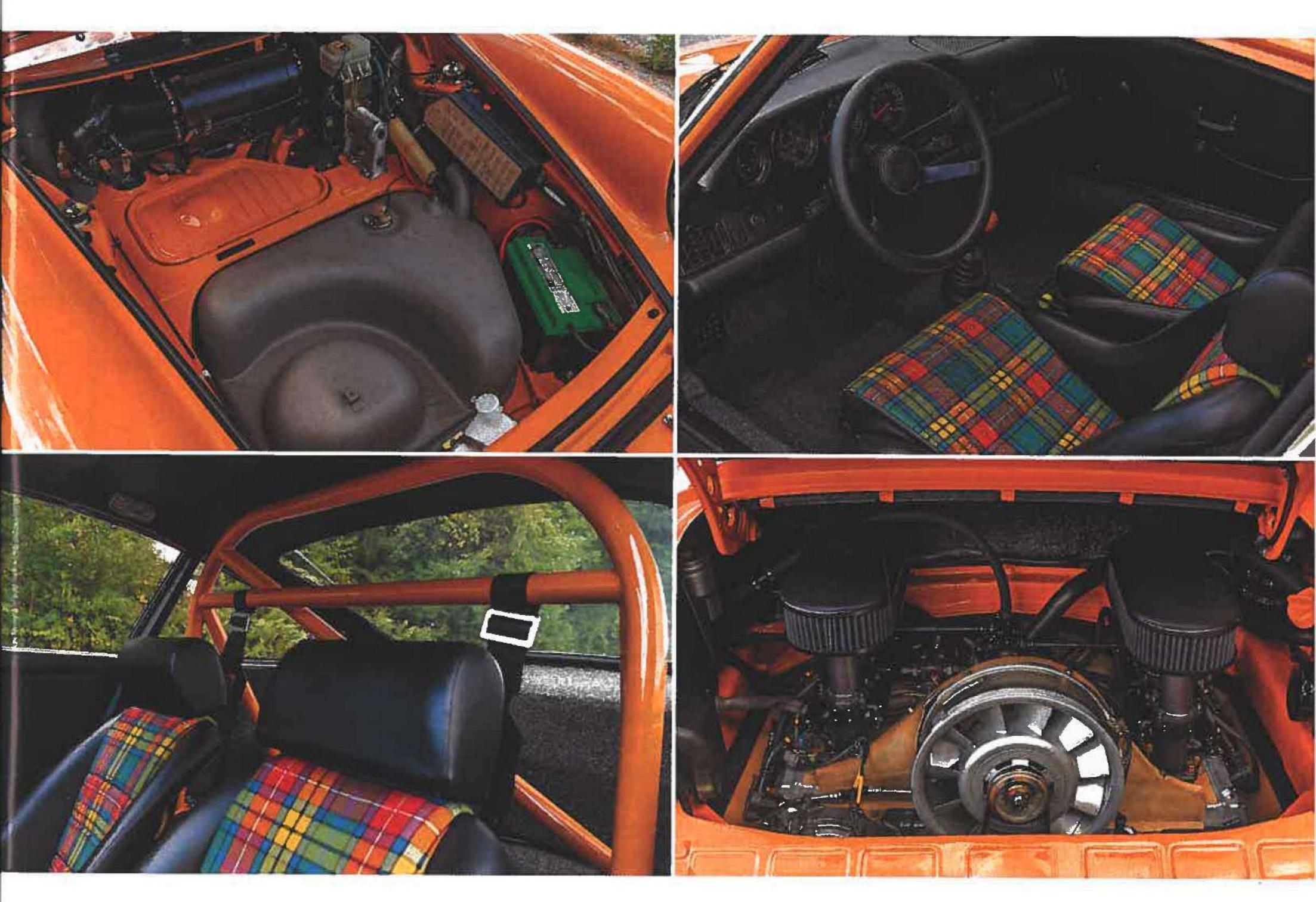
Bahama Yellow RSR Project car. A pristine 1987 911 Carrera 3.2 was sourced, and the rebuilding process began. The engine was enlarged to 3.4 liters, fitted with RSR racing cams, and rebuilt. However, just as the flat-six was ready to go into the car, the customer decided to add Kinsler ITBs (individual throttle bodies) with a Motec management system to the engine.
