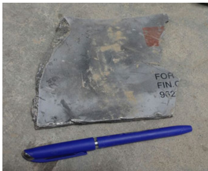
A remnant of what appears to be a guided bomb unit found at the scene of the attack on Al-Khansa Girls' School. The marking "962" appears to be the initial digits of US defense contractor Raytheon's CAGE number (96214), likely identifying Raytheon as the manufacturer of the part.
