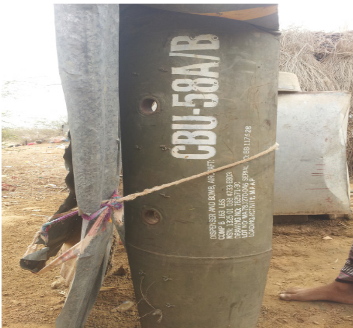
A US-made CBU-58 cluster bomb casing recovered at the scene of the attack in Bani Haddad village. The CBU-58 cluster bomb disperses about 650 BLU-63 submunitions widely and indiscriminately.
