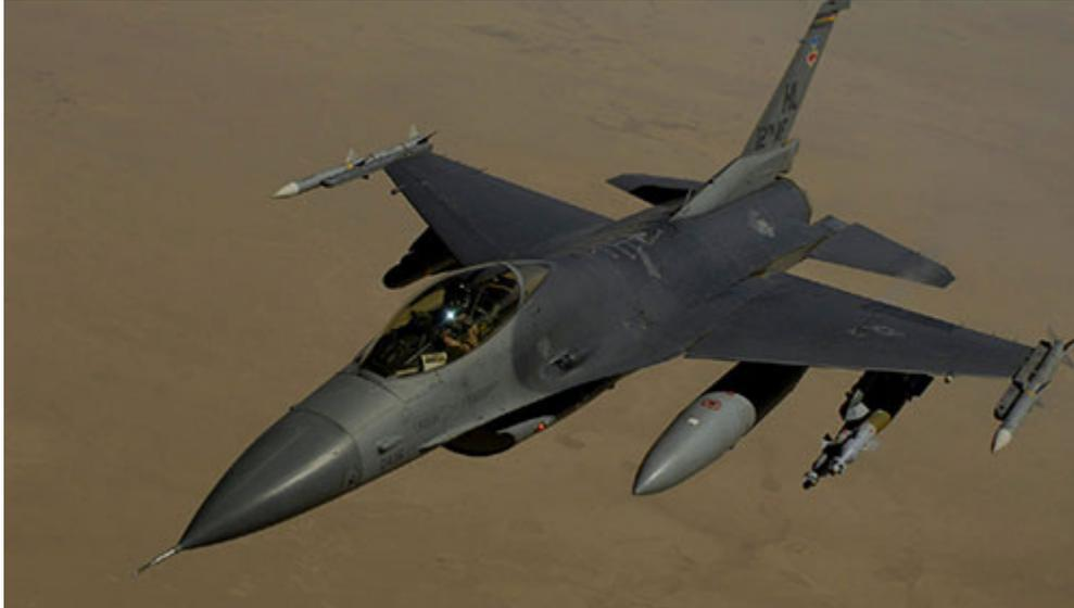
The F-16C is a cost-effective multi-role fighter aircraft designed for air superiority. With features such as a frameless bubble canopy for enhanced visibility, a seat which helps reduce the effects of g-forces on the pilot, and a state of the art flight control system, the F-16 is one of the most common currently operational military aircrafts, with over 4500 F-16 aircraft in operation around the world.
