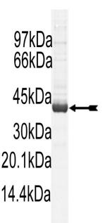
SDS-PAGE and Coomassie Stain: Purity was assessed by SDS-PAGE and Coomassie blue staining using 3µg of TAO1, active.
