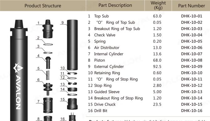
**Products features:** Valveless air distribution hammer, more reliable,. Good sealability, no water and cuttings entering into hammer in water exists drilling.
