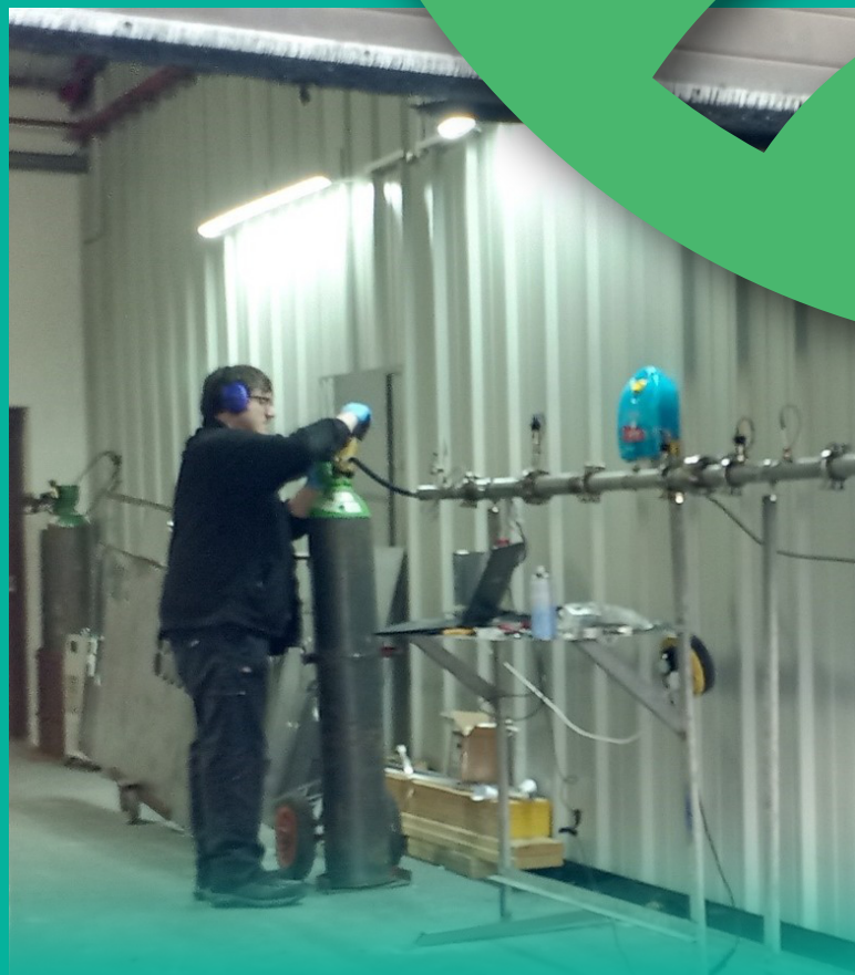
Figure 2: Croft Filters' custom-built flow test rig, designed to simulate high-pressure gas
