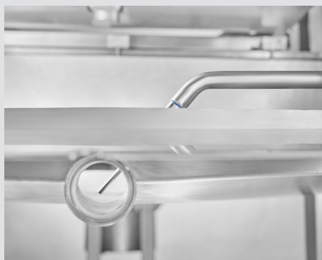
Boundary temperature control Temperature sensor linked to control system at boundary
