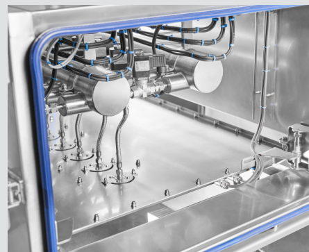
Heated drip plate No water ice falling into the product
