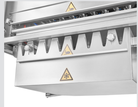
Bottom exhaust To avoid contaminated condensate
