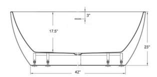
Note: ALL MEASUREMENTS ARE IN INCHES & HAVE TOLERANCE OF +/- 1/4"
